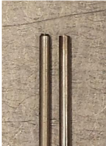
Figure 33: Chamfered [L] and Blunt [R] Fuel Tube Comparison
